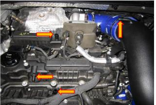
4. Make sure the two draining points at the bottom of the catch tank are fully tightened. Use a 17mm spanner to do this.
