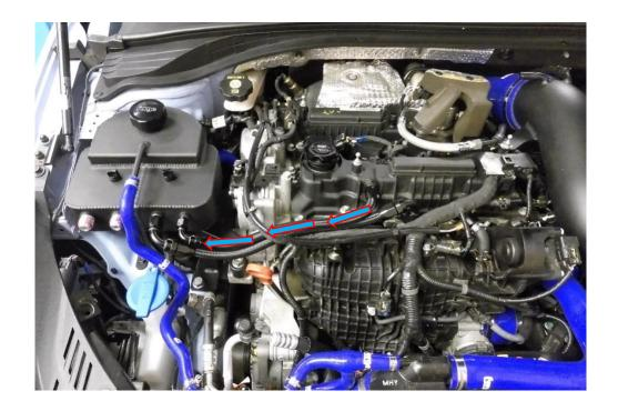
12. Take the longest hose from the kit and run the hose as shown in the picture below. Unclip the wiring loom to the injector behind the oil cap, this will allow you to run the hose underneath it, then re connect the loom. Use a 25mm spanner to tighten the AN-10 fitting and a 7mm socket for the hose clamp at the other end of the hose.
