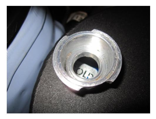
**15.** Take your original coolant cap and screw onto the Forge expansion tank. Once fully tightened place the Forge alloy cap over the OE cap line it up and fix into position with the grub screw.
