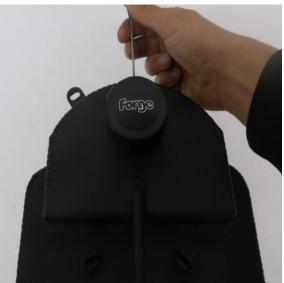
. Do a final spanner check on all your fittings and re fit the engine cover. Your installation of FMCT-5 is now complete.
