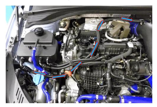
13. The last hose to be installed is another AN-10, run the hose as shown in the picture. As in step 8 the breather end has a push fit machined boss which is secured in place with a M4 fastener. Use 26mm spanners to tighten.
