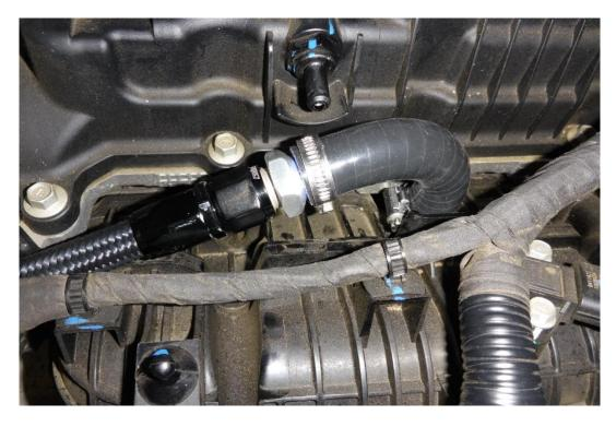
11. Attach the AN-6 fitting of the smaller hose to the catch tank and run the hose to the rocker cover as shown in the picture below. Use a 17mm spanner to tighten the AN-8 fitting and a 7mm socket to tighten the hose clamp on the breather end of the hose.
